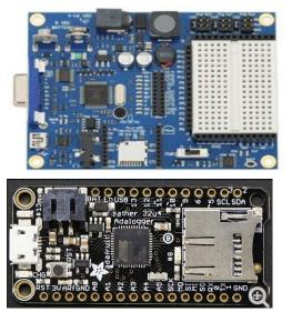
Figure 15 - Propeller and Feather 32u MCU [47]
