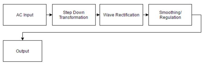
Figure 37 - Block level diagram for the AC/DC converter [70]
