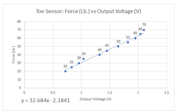
Fig. 48 - Force vs Voltage of Top Sensor [85]
