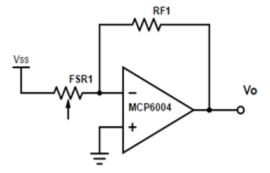
**Fig. 29 Inverting op-amp configuration**. [63] FSR1 is the force sensitive resistor and RF1 is the reference resistor.
