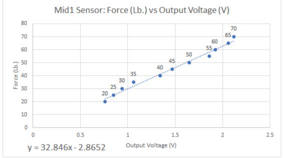
Fig. 49a - Force vs Voltage of Mid Sensor (1) [86]
