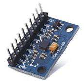
Fig. 32 MPU-9250 gyroscope-accelerationmagnetometer combo. [65]
