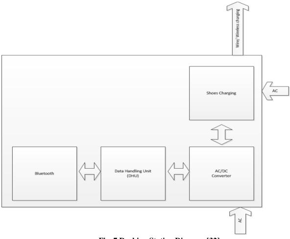
Fig. 7 Docking Station Diagram [32]
