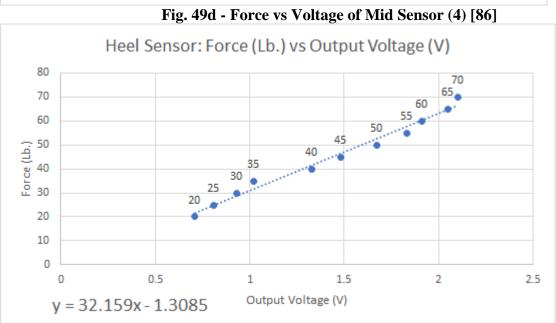
Fig. 50 - Force vs Voltage of Heel Sensor [87]
