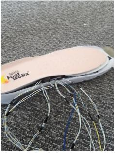
**Fig. 44 - Shoe Wires Assembly [81]** The blue pucks visible in the picture is a small disk that was 3d printed to help distribute the weight evenly across the sensing area. The shoe was put together using shoe glue and was set to dry over a 48 hours. See fig 45.[82]
