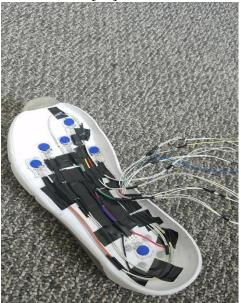
**Fig. 43 - Bottom Shoe Sensors Assembly-1 [80]** The figure 44 shows the material that will be placed on the this portion of the shoe. [81]
